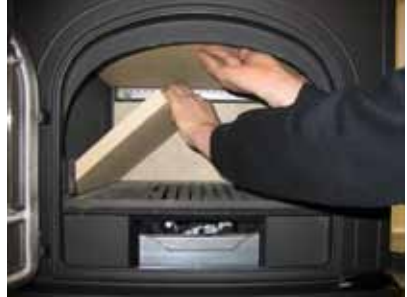
b. Lift the lower baffleplate a bit and hold in that position. Carefully lift and remove the two side bricks.
