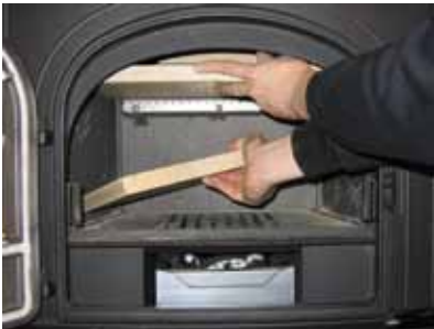
c. Remove the firebrick from the back-wall
