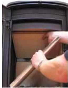
3. Tip the other side brick and remove it from the fire chamber.
