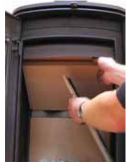
4. When the side bricks are removed the bottom baffle is lowered and lifted out of the fire chamber.
