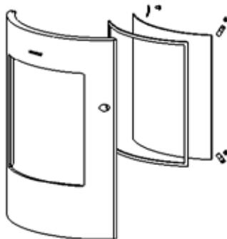
1. When you open the door, you will find two hinge pins, one in each hinge. Remove the two hinge pins, lift the door off the hinges and place it face down on a sheet of cardboard or other nonabrasive fabric.
