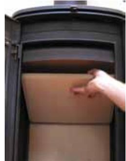
5. The upper baffle is removed from the brackets and lifted out of the fire chamber.
