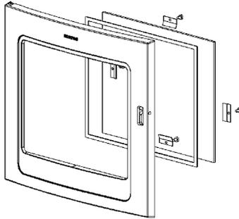
2. Unscrew the 4 bolts that secure the glass. (In the event that a bolt sheers off when being unscrewed, remove the remaining body of the bolt by drilling down its centre with 1/8 inch high speed steel drill bit. Smaller drill bits may be successful, but do not use a larger bit. Make sure the bit stays away from the edges of the bolt - this may damage the thread in the cast iron).
