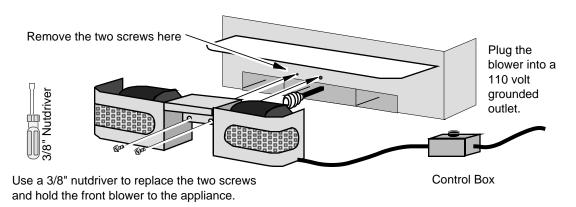
2. Plug the power cord running from the control box into a grounded 110 volt electrical outlet.
