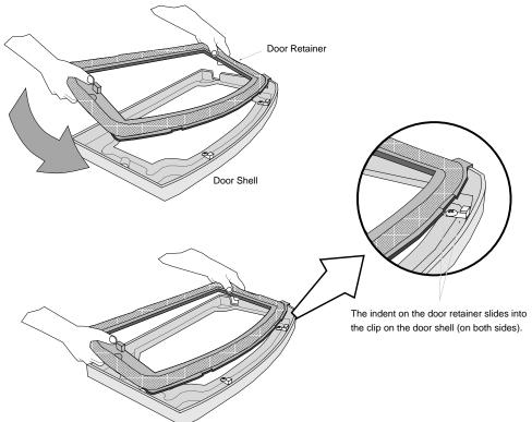
3 Attach the retainer to the shell following the directions below.
