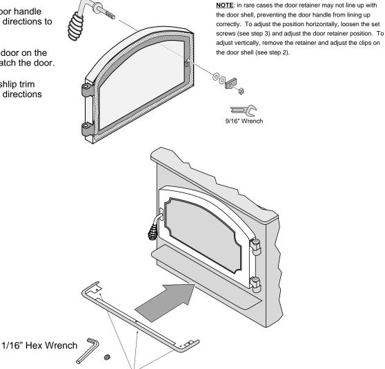
Slide the ashlip trim into place then tighten the three set screws on the bottom of the ashlip to secure.
