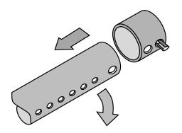
Slide the air tube to the left, swing it down and remove from the firebox.
