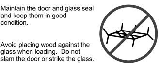
Do not use a grate or other device to elevate the fire off of the firebox floor. Burn the fire directly on the bricks.
