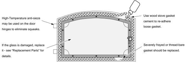
The door latch should pull the door against the face of the stove (but not so tight as to not allow full handle rotation). If the latch requires adjustment, follow the directions below.
