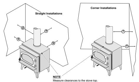
Minimum Clearance Reduced Clearance (See the illustration above) Connector Sidewall to stove 13" В Backwall to stove 9" С 7-1/2" Cornerwall to stove D 21-1/2" Connector to sidewall Ε Connector to backwall 11-1/2" Connector to cornerwall 16-1/2"
