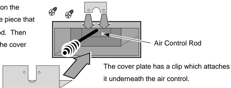
The cover plate has a clip which attaches it underneath the air control.
