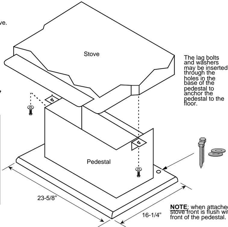
The lag bolts and washers may be inserted through the holes in the base of the pedestal to anchor the pedestal to the floor.
