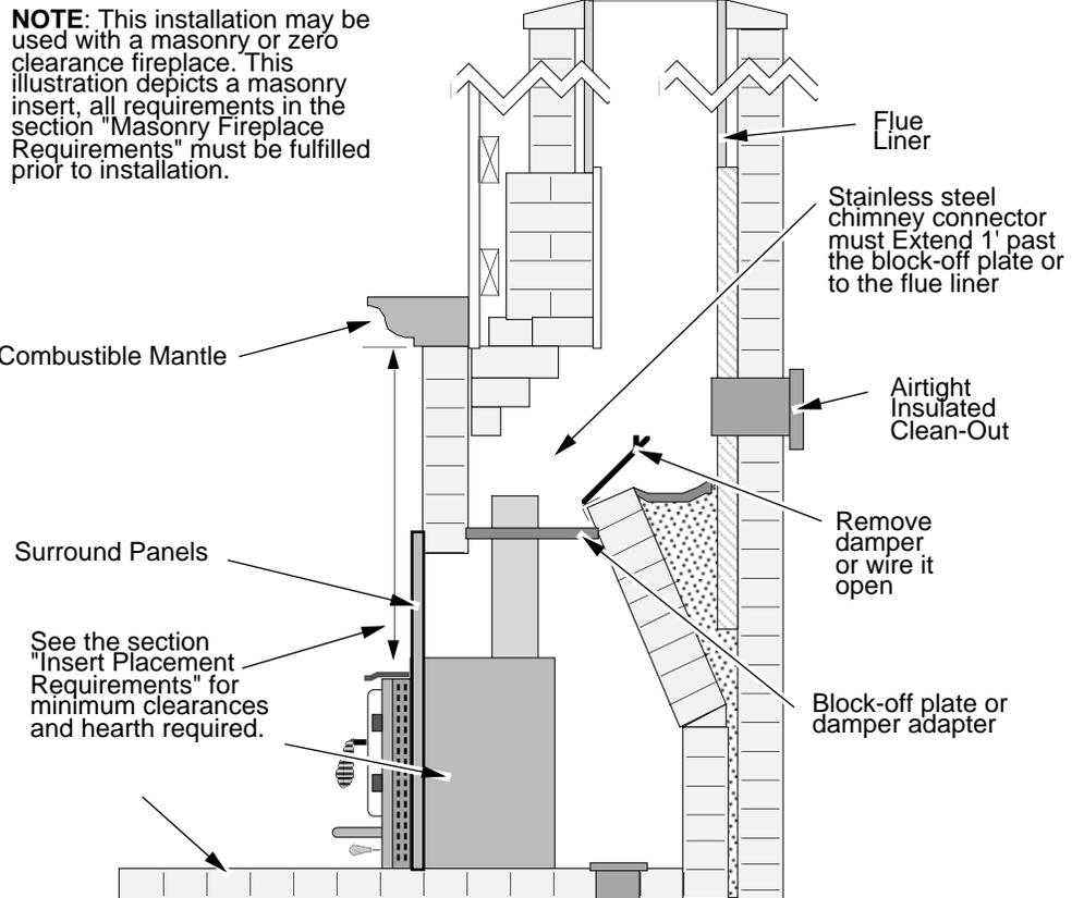
**NOTE:** This installation may be used with a masonry or zero clearance fireplace. This illustration depicts a masonry insert, all requirements in the section "Masonry Fireplace Requirements" must be fulfilled prior to installation.
