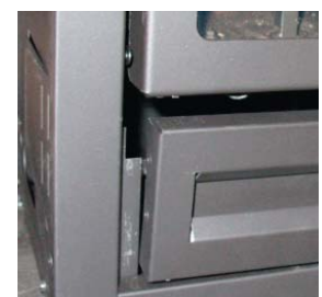
Installation of lower Louver/Flush Panel
