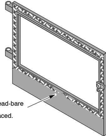
Severely frayed or thread-bare gasket should be replaced.
