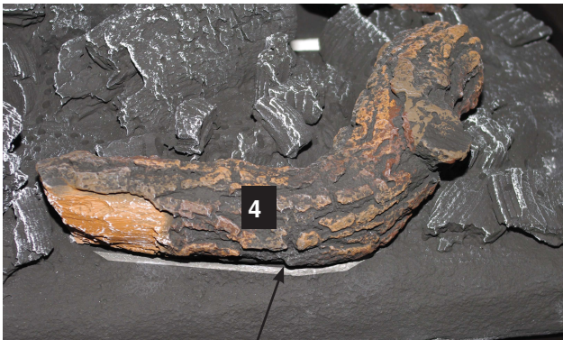
Ridge in burner tray (highlighted)
