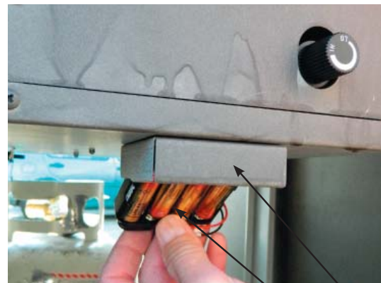
Battery compartment Battery pack
