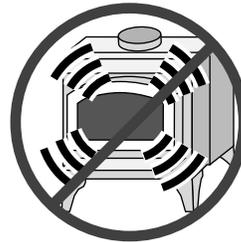
Do not make any changes to the appliance to increase combustion air.
